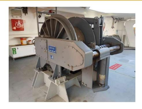
1x 12.5 ton Towing Winch, 51 ton brake 1x 8.7 ton Towing Winch, 35 ton brake 1x 10m Deck Crane 3T/6T 1x 10 ton Lifting Platform of 5mx3.8m
