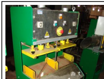
#26: Press for assembling wedges / soles
